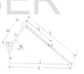
Figure 4. The Schematic diagram of the Offset Slider Crank
