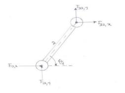
Figure 5. Free-body diagram of link 2.
