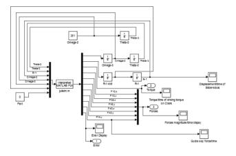
Figure 8. Full Dynamic Simulation of Offset Slider Crank
