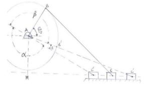
Figure 1. Offset Slider Crank Mechanism
